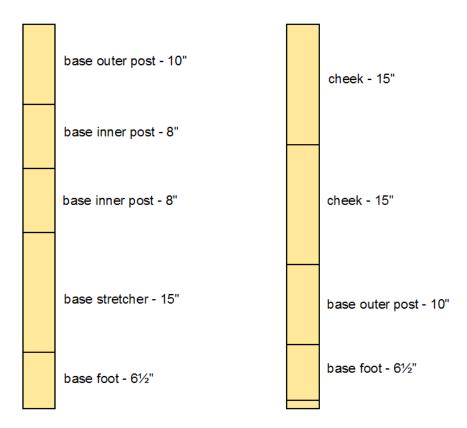
You can do this easily using a miter-box and a backsaw. If you have access to a power miter saw, table saw, or radial-arm saw, you can use that instead.
